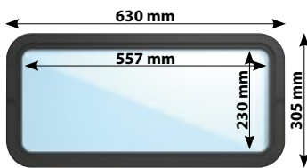
Rounded corners (r=60 mm), excellent insulative value
