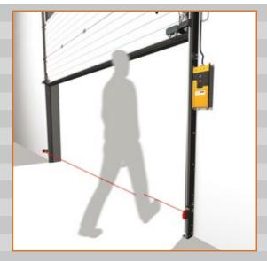
rail. If the beam between the transmitter and the reflector/receiver is broken, a signal is sent to the motor to stop and reverse the movement. While the reflector system is sensitive to dust and moisture, this is not the case for the receiver model.
